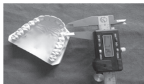
Figure 2: Measurement of buccolingual dimension of canine with digital calliper (0.01 mm calibration).
